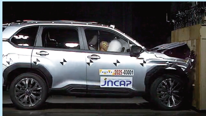
A full-wrap collision test
