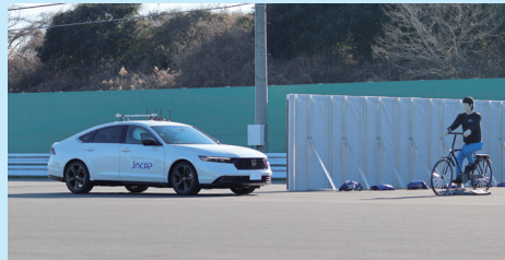
A test of collision damage reduction brakes
