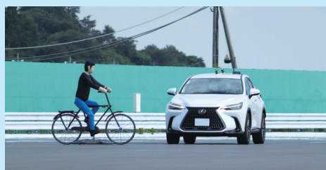
Collision damage reduction brake test
