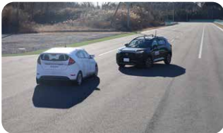
AEBS intersection : car to car (right turning-omcoming)
