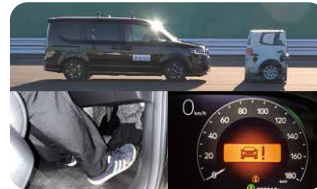
Pedal misapplication prevention device
