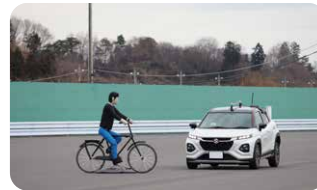
AEBS to avoid collisions with a bicycle
