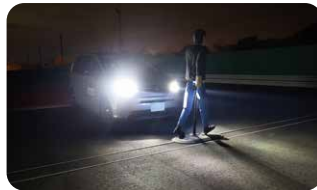
AEBS to avoid collisions with a pedestrian (at night)
