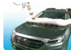
Pedestrian head protection performance test
