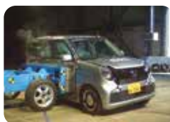
Side collision test
