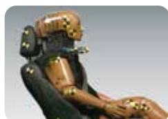
Performance test for neck injury protection in rear-end collision
