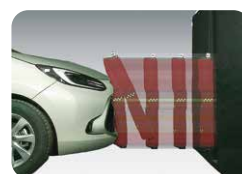
Pedestrian leg protection performance test
