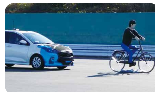
AEBS* to avoid collisions with a bicycle
