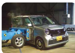
Side collision test
