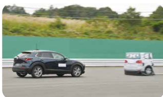
AEBS* to avoid collisions with a car
