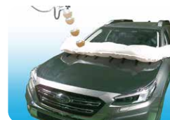
Pedestrian head protection performance test
