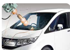
Pedestrian head protection performance test
