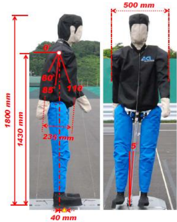
(a) Movable Dummy Specifications
